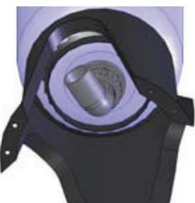
Connect the Union fitting to the inlet bushing (bottom)
