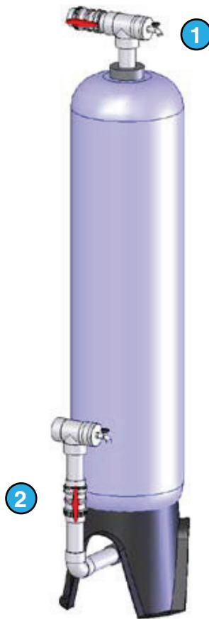
1. Connect a hose to the hose babb on the outlet of the tank. Run the hose to a drain.
